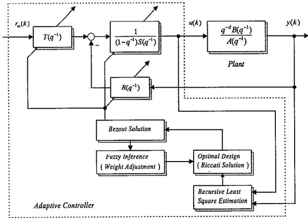
Fig.2. Block diagram of proposed adaptive control system.
