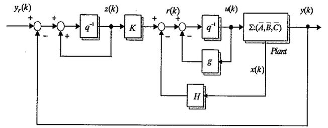
Fig.1 Type-1 optimal servo system having one sample delay.
